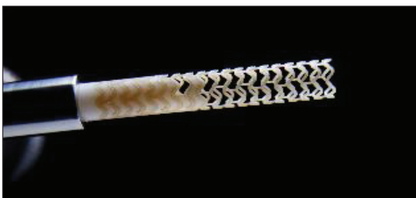
Figure 2. Laser-cutting of Fantom from a Tyrocore tube.
